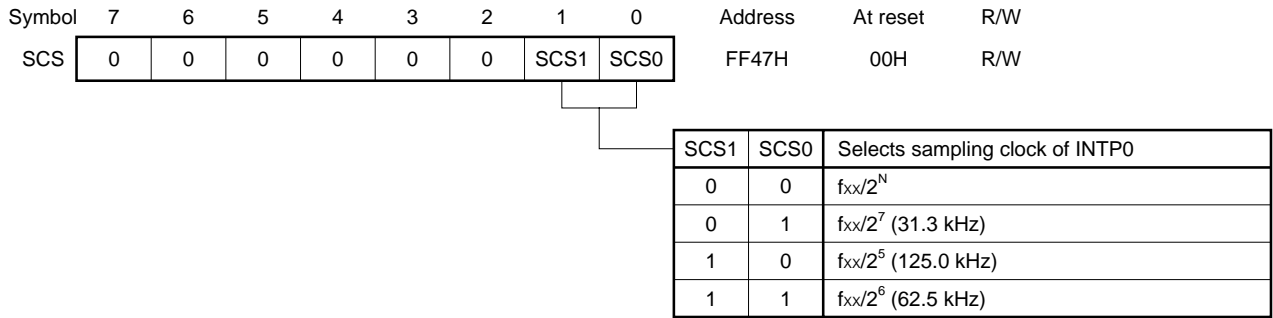
Figure 5-10. Format of Sampling Clock Select Register ( \mu PD78098, 78098B subseries)
