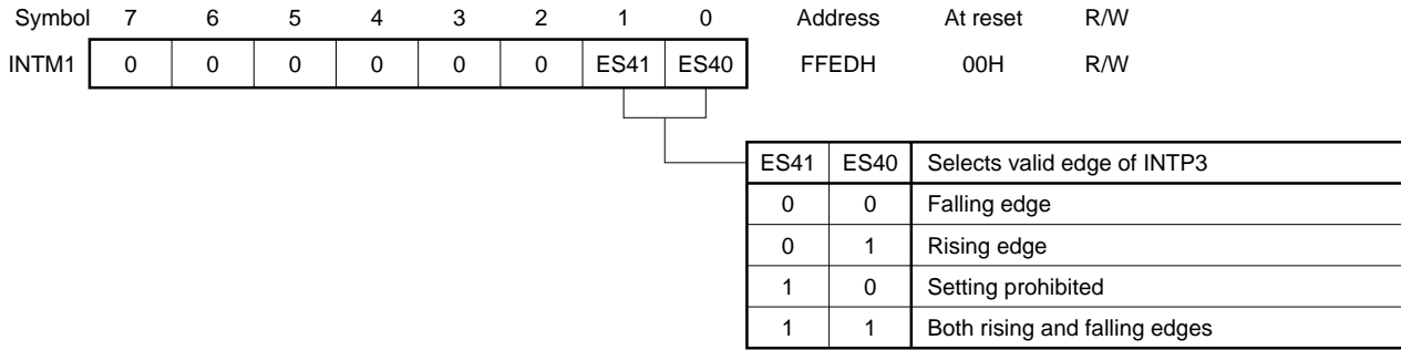
Figure 9-7. Format of External Interrupt Mode Register 1 ( \mu PD78083 subseries)
